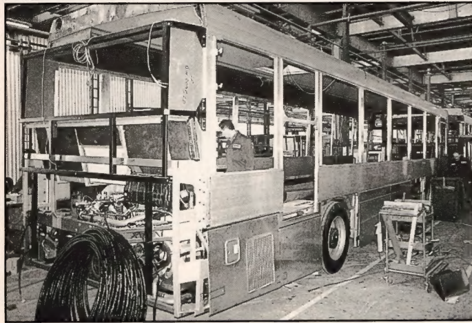
A Mercedes Benz 0405 mounted Prisma taking shape on one of the production lines.
